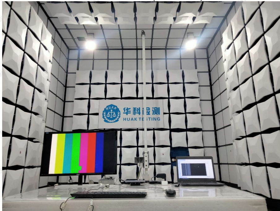
Radiated Emission (1GHz-6GHz)
